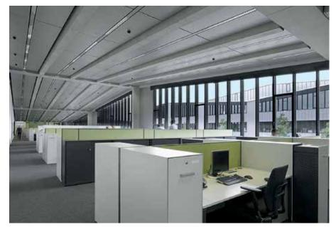
Despite the large glass front panels, Zehnder heating and cooling ceiling sails guarantee a comfortable indoor climate. At the same time, thanks to their noise-insulating effect, they also ensure comfortable acoustics.
