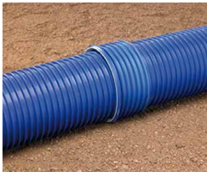
4. The pipes should be fitted to the sleeve base plate. Make sure there is no gap between the pipe end and sleeve base plate. Directional changes of \leq 4^\circ are achieved by a joint deflection at \text{Ø } 200 \leq 315 .
